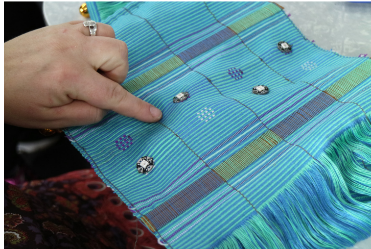
Figure 3: LEDs sewn onto a tung (hand-woven cotton banner). Photo credit: Kay Sneddon, Nelson.
